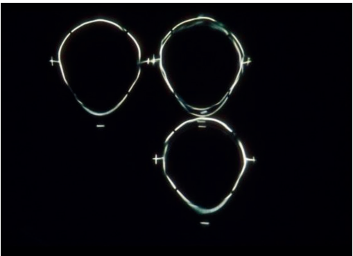
Figure 4. Bausch & Lomb one-position keratometer showing mire distortion.
