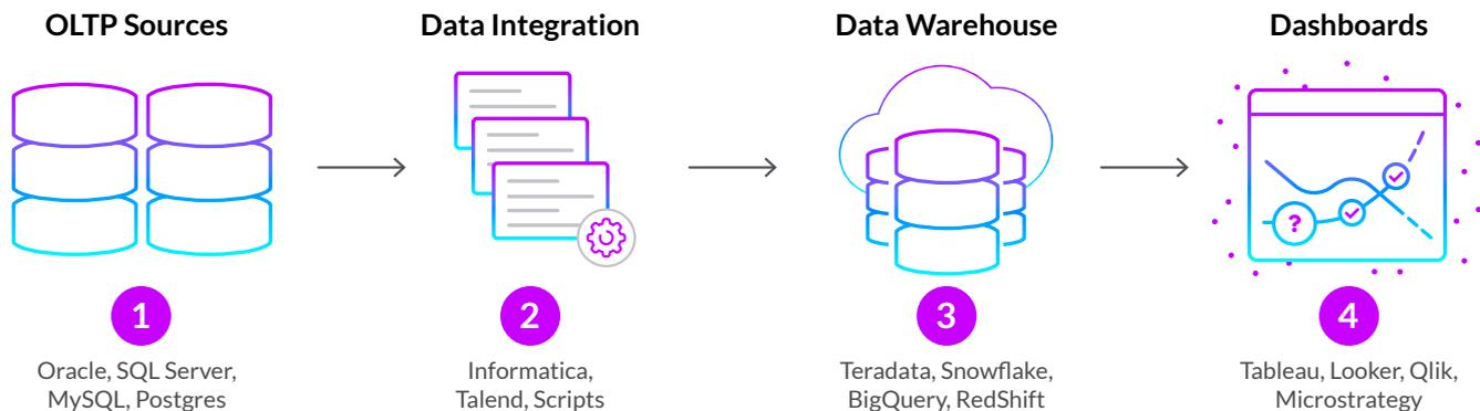
Figure 1: Common data flow for analytics and data warehousing
