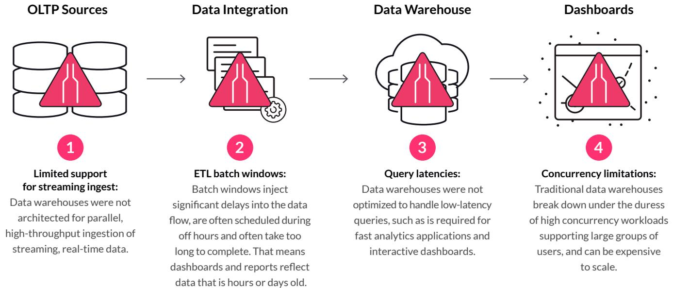
Figure 2: Common bottlenecks associated with the data warehousing flow
