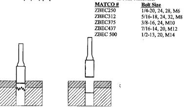
OP 2 - Set ZBCD5 - provides 5 specialty angle ground burs for use after OP 1, will properly locate broken bolts center point providing greater ability for the drilling operation to drill in center.
