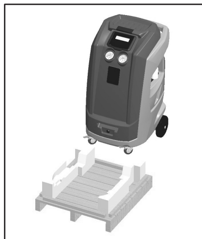
Fig. 12: Lowering unit from the pallet
