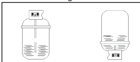
Fig. 13: Virgin refrigerant cylinder tank types
