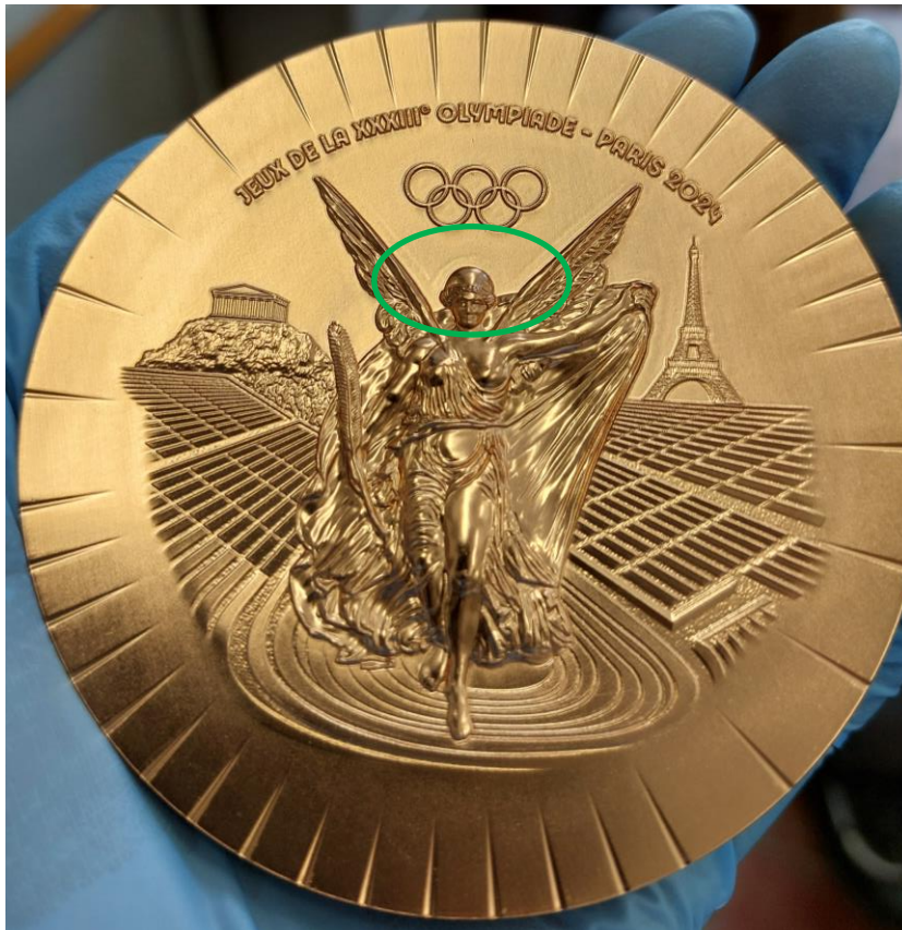
Light halo close to the head of the goddess due to the varnish process
