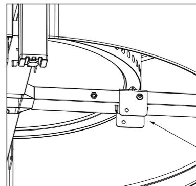
*Note location of fire pit support bracket when installed correctly.*
