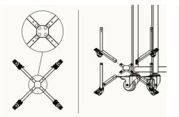
**Step 1:** Match the corresponding numbers from the lower legs to the cross-member bracket, and slide each of the lower legs onto the cross-member bracket.
