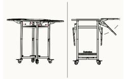
**Step 7:** Use (4) step screws in the lower hole positions to secure the shelf to the upper legs.
