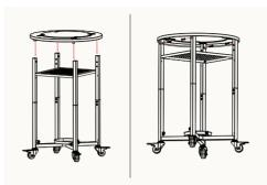
**Step 5:** Align the top shelf into place over the upper legs. Secure the top shelf into place using (4) screws and washers.
