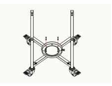
**Step 2:** Connect the propane tank base to the crossmember bracket using (4) screws and (4) washers.
