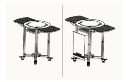
**Step 8:** Locate the side of the Cart with (2) magnets facing outwards on the bottom legs. Slide the Solo Stove branded logo panel into each hole located below the middle shelf.
