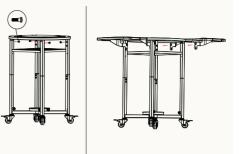
**Step 6:** Loosely attach a step screw into each upper leg in the top holes position only.
