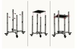
**Step 4:** Loosely attach (4) screws and (4) washers into the appropriate holes on the upper legs. The screws should be facing in towards each other.
