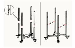
**Step 3:** Match the corresponding numbers from the lower legs to the upper legs. Attach the appropriate upper leg to the lower legs using (2) screws and (2) washers for each leg.
