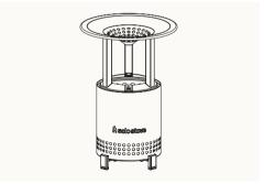
Do not use the heat deflector if the fire level is consistently near or above the level of the bottom of the cone of the deflector. High fires will reduce the effectiveness of the heat deflector.
