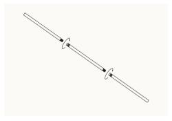
Twist the pole sections together, using the piece with threads on both ends as the middle section.
