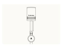
Clip the snuffer cap and snuffer holder onto the top section of the pole and position it about six to nine (6-9) inches below the fuel canister assembly.
