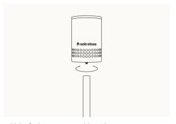
Add the fuel canister assembly to the top of the assembled pole.
