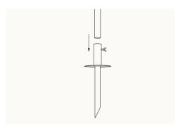
Attach the ground stake to the bottom portion of the pole, positioning the tension screw towards the rear. Tighten the tension screw so that it is firmly connected to the pole.
