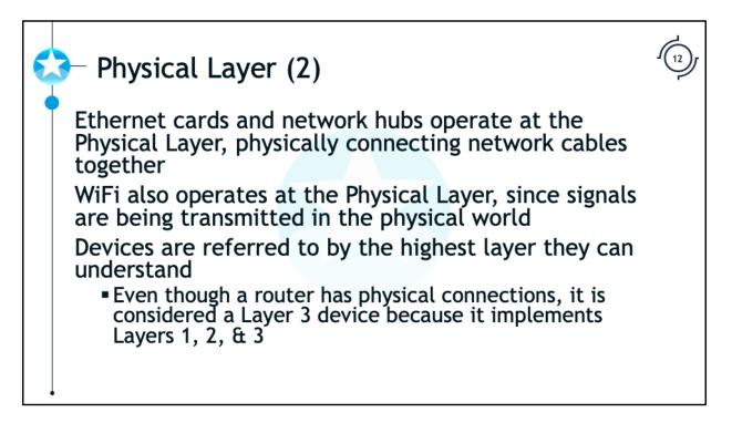
Network cables, cards, and hubs all operate at the Physical Layer. A hub operates at the physical layer by electronically connecting the wires of multiple network cards. WiFi also operates in the Physical Layer even though it doesn't involve physical cables, since it uses radio signals to transmit data through the physical world.
