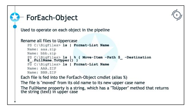
The ForEach-Object cmdlet is incredibly powerful. Linux has a command similar to this, xargs, but it is not nearly as powerful. If multiple commands are nested it is quite difficult to write (and read) the xargs command. For example, if we wanted to read the contents of a csv file which contained a list of large files, then move those files if they are still too big:
