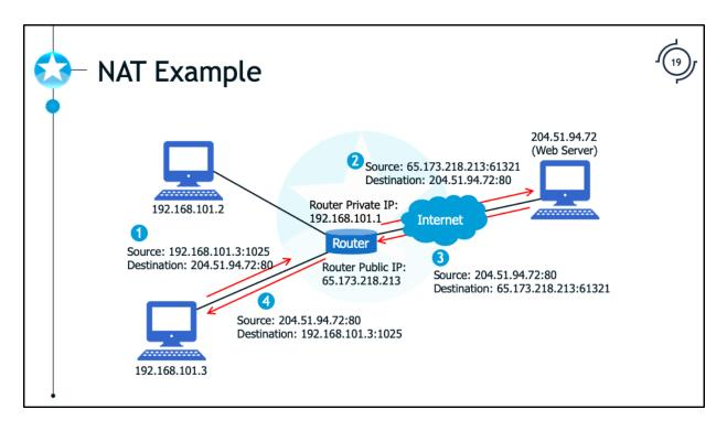
The above diagram represents a typical home network using NAT (specifically, PAT/IP masquerading). The computers on the home network (left) are on the private IP range 192.168.101.0/24, and are connected to the Internet through a NAT-enabled router. The router's private (internal) IP address is 192.168.101.1, and the router's public (external) IP address is 65.173.218.213. Let's say that the computer at 192.168.101.3 would like to fetch a web page from the web server at 204.51.94.72.
