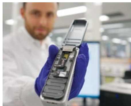
The MinION sequencer allows researchers to sequence DNA on their laptops.
