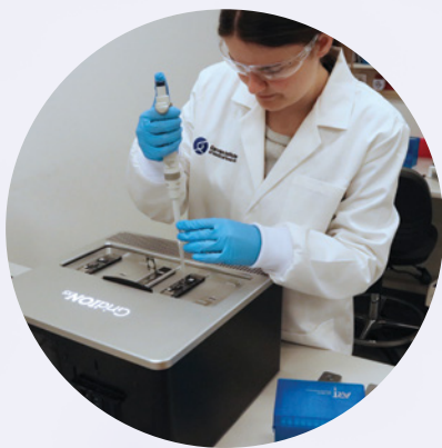
Garvan's Jillian Hammond loads an Oxford Nanopore GridION flow cell.
