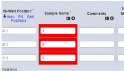
Figure 30: Premix SEQ & Fragment Analysis screen with errors highlighted red
