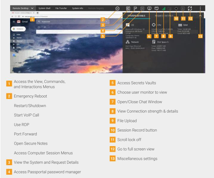
The Remote Viewer is the remote access tool launched by the technician to access the end-user's desktop.
