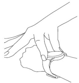
If the InBodyWATCH cannot come into full contact with your wrist, fasten the watch tighter or move it further down your arm until the electrodes are in full contact with your skin.
