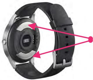
The bottom electrodes must touch your wrist completely.
