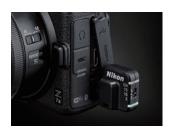
\*1 Radio-controlled AWL with the Z 7II and SB-5000 units requires the WR-R10 or WR-R11b Wireless Remote Controller.
