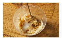
**Tip:** In case your joints are not as tight as you would have liked, you can make your own wood filler to fill any voids. Simply mix some sawdust and glue until you have a cookie dough-like texture. Immediately scrape it where needed, let it dry, then sand the excess.
