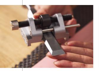
**Tip:** If you run your finger underneath the blade, the edge will feel a little rough from the steel that has folded over. This is called a burr and needs to be removed after the secondary bevel has been polished. However, don't worry if you can't feel this burr.
