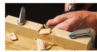
**Tip:** Chisel down to the baseline by paring across the grain, about halfway across the width of the piece. If you cut all the way across the workpiece, there is a chance that you will experience tear-out. Pay attention to the direction of the grain; you may need to take slightly angled cuts in the direction of the grain if it runs out.
