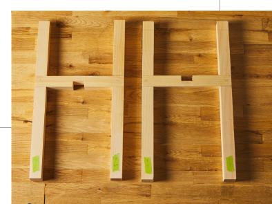
**Tip:** Apply and spread the glue with a stick or your finger. There should be a thin film on the face grain. Don't worry about glue on the end grain as that is not the structural part of this joint. You should see glue bubble out, but if it flows out, you are using more glue than you need. Too much glue will cause the joint to shift as pressure is applied.
