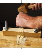
I. Unclamp the piece of wood, turn it end for end and re-clamp it. Repeat the previous steps to incise and cut the shoulder line on the other side of the waste area.
