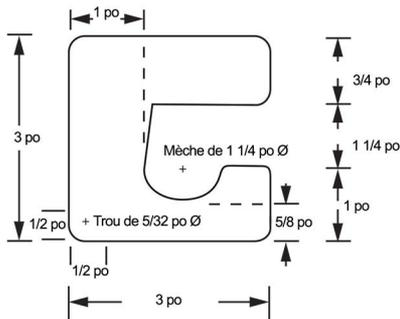
Figure 2 – Support pivotant
