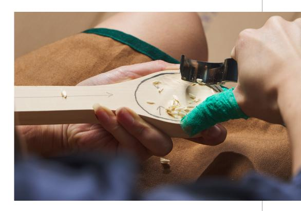
c. Pull the knife away from the pencil line towards the center of the bowl and start scooping the first shallow layer of wood out of the bowl. Work against the grain. While you will need to do more than scrape the wood, watch that you don't dig too deep.
