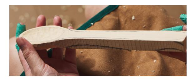
b. Carve the edges away, moving down from the bowl and up along the handle in alternating strokes, and around all four sides of the handle.
