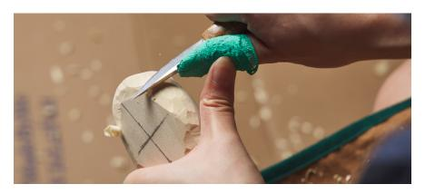
**Tip:** Carve the back of the bowl to match the shape of the bowl itself. For example, a deep bowl could have a rounder back, while a shallow one could have a flatter back.
