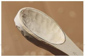
b. Carve the sides from the front to meet the back of the bowl, taking only a thin slice of wood off all the way around.
