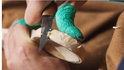
**Tip:** Refrain from carving the sides by coming forward from the back because you have already carved away the inside of the bowl, and there is little or no wood to support the edge. You can easily mar the front of the spoon by chipping out a piece, especially at the top where you are working in end grain. Keep in mind that you will also be sanding these areas later, so paring just enough to shape the outer rim might help prevent tear-out in this area.
