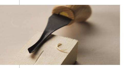
The palm parting tool has two straight cutting edges that make a sharp 1/4" wide V-shaped groove set at 70°. This tool is effective for carving grooves, lines and channels. Use it for adding details and texture, as well as for outlining design elements to obtain the desired shape and depth.
