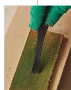
**Note:** When you notice that stropping no longer has an effect on the blade's edge, it will be time to sharpen your tools with the wet/dry sandpaper and the scrap piece of wood, and then follow up with stropping with the honing compound and leather strop, as described above. For a tutorial on using sandpaper as sharpening media, please watch our **Film & Paper** video on our **Sharp-Net** page on our website.
