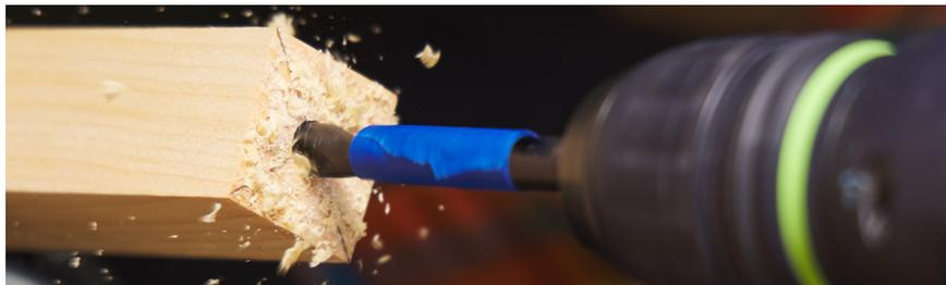
**Tip:** To ensure proper alignment of the parts, be sure to drill the holes into the post as straight as possible. Adjust the drill by eye so that it is in line with the post. Maintaining up and down alignment is harder, unless your drill has an integral level.
